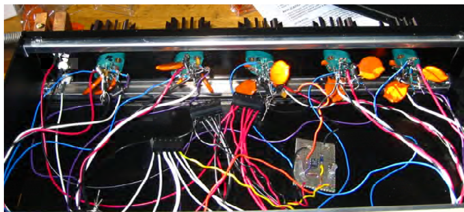
Figure 2.16: Photo of the inside of the high voltage box. Five amplifiers are soldered directly to the sockets for the amplifiers.
