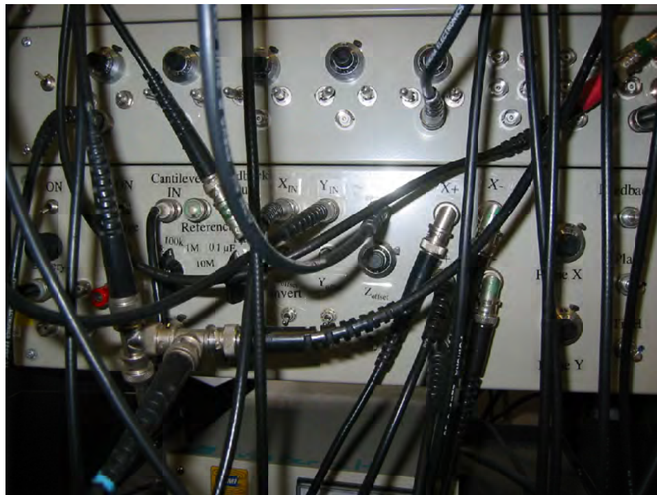
Figure 2.10: Photo of the XYZ box, below the voltage reference box, with all the regular BNC connections.
