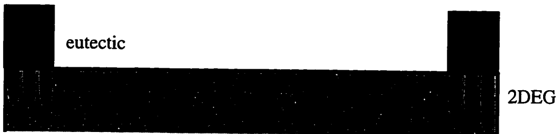
Figure 3.2 Au/Ni/Ge contacting process. (a) Openings ("windows") are defined in a resist layer where contacts are desired; (b) after evaporation and liftoff, sequence of metal layers remains where openings were; (c) after annealing, metal forms eutectic and tendrils penetrate semiconductor to contact 2DEG.
