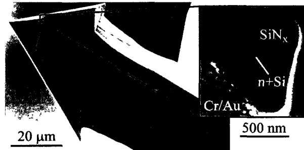
Figure 6.3: Scanning electron micrograph of a typical coaxial AFM probe for DEP imaging and manipulation.[78] The inset shows a magnified view of the coaxial electrodes in which the triangular inner conductor is visible.[79]
