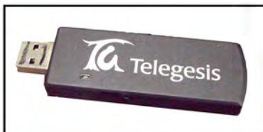
Figure 8.8: Zigbee USB transceiver based on the EM250 SoC.
